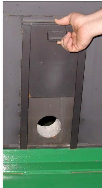
Access Door for Lighting
