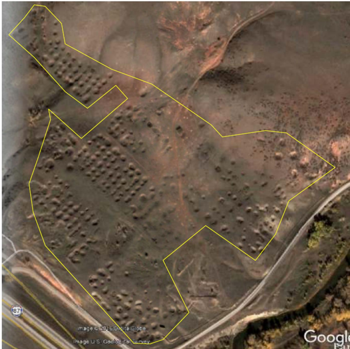
AREA 1 MINE SUBSIDENCE FROM UNDERGROUND MINING OF THE CARNEY NO.44 MINE. MINE DEPTH IN NOTED SUBSIDENCE AREA RANGED FROM 50 TO 160 FT. (ADD_D5-4_EX_1_OVB_ISO_R1)
