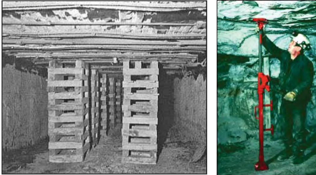
Fig 1.1.2e – Crib blocks (Darling 2011) and Jack Support (Gilmore-Kramer)
