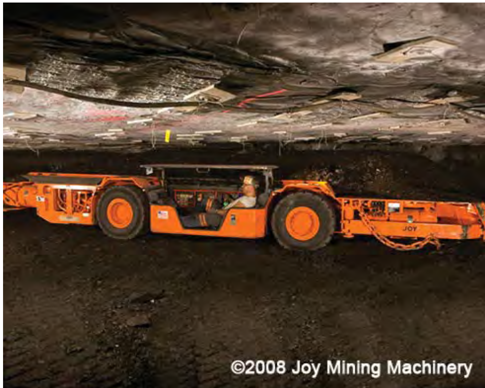
Fig 1.1.2d – Shuttle Car (Joy Mining Machinery Website)
