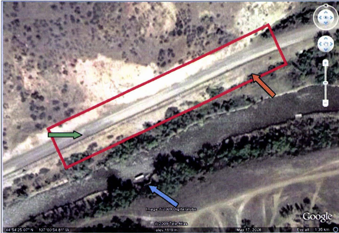
Photo 3. Aerial photograph of immediate project area. Red line represents an approximate project APE. Green arrow identifies where main haul way crosses under county road. The darker blacktop patch can be seen on the county road. Orange arrow identifies approximate location of the smaller, eastern mine entry. Blue arrow identifies Carney trestle abutments in Tongue River.
