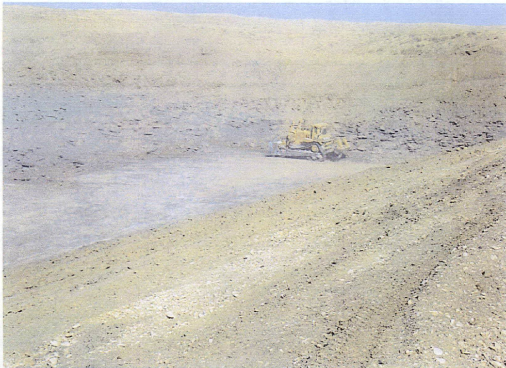
Photo 1 (top) looks generally west showing a D10 dozer moving overburden near Cut 18 as shown on the AR Map. Photo 2 (bottom) looks southwest and shows where the mined out pit void has been bridged to allow scrapers access to a topsoil stockpile opposite the parked scraper in the photo. The topsoil salvage area is located in upper photo right.
