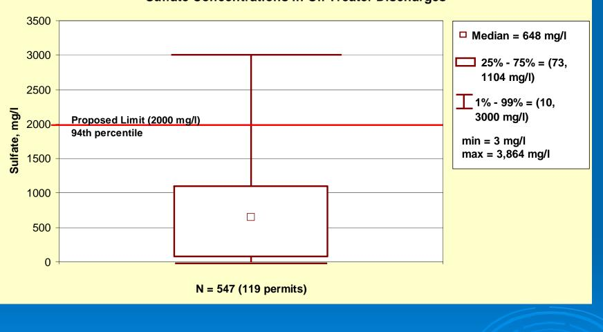
Sulfate Concentrations in Oil Treater Discharges
