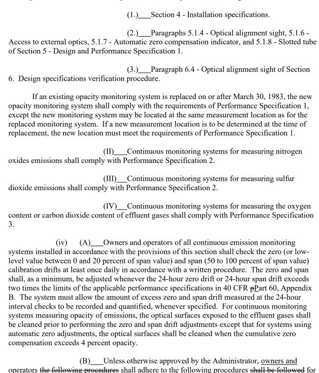
continuous monitoring systems measuring opacity of emissions. Minimum procedures shall include a method for producing a simulated zero opacity condition and an upscale (span value)
