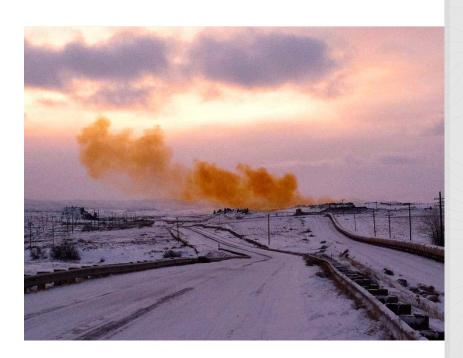
Today, blasting at the Rosebud Coal mine owned by Western Energy Company created clouds of hazardous gases which is a common occurrence in coal strip mining. The actual meteorological conditions at the time of firing the blast will have a significant impact on the fume
