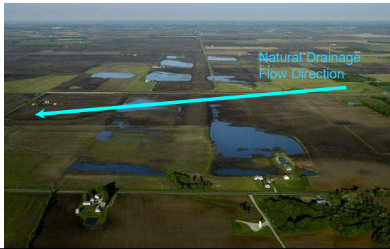
Drainage problems from chain pillars between subsidence troughs
