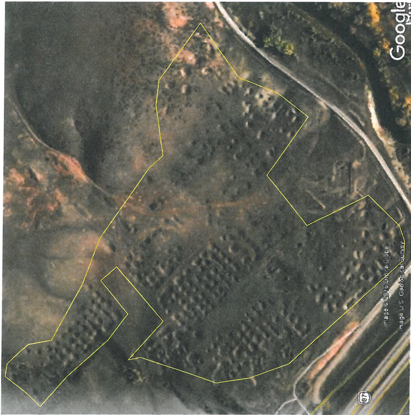
FIGURE 7.2 AREA 1 MINE SUBSIDENCE FROM UNDERGROUND MINING OF THE CARNEY NO. 44 MINE. MINE DEPTH IN NOTED SUBSIDENCE AREA RANGED FROM 50 TO 160 FT. (ADD_D5-4_EX_1_OVB_ISO_R1)
