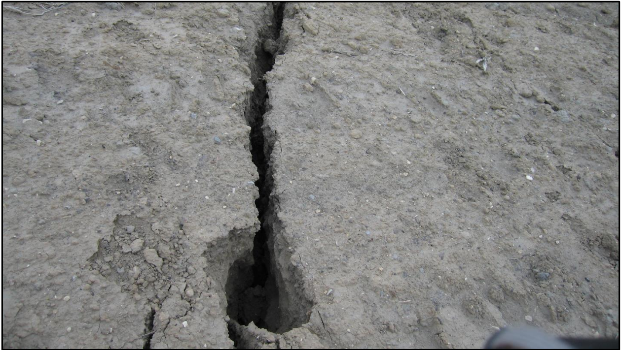
Photo 9 (above) looks north-northwest across a regrade area on the side of the north pond area where a series of tension cracks have developed. Photo 10 (below) is a close-up of a tension crack.
