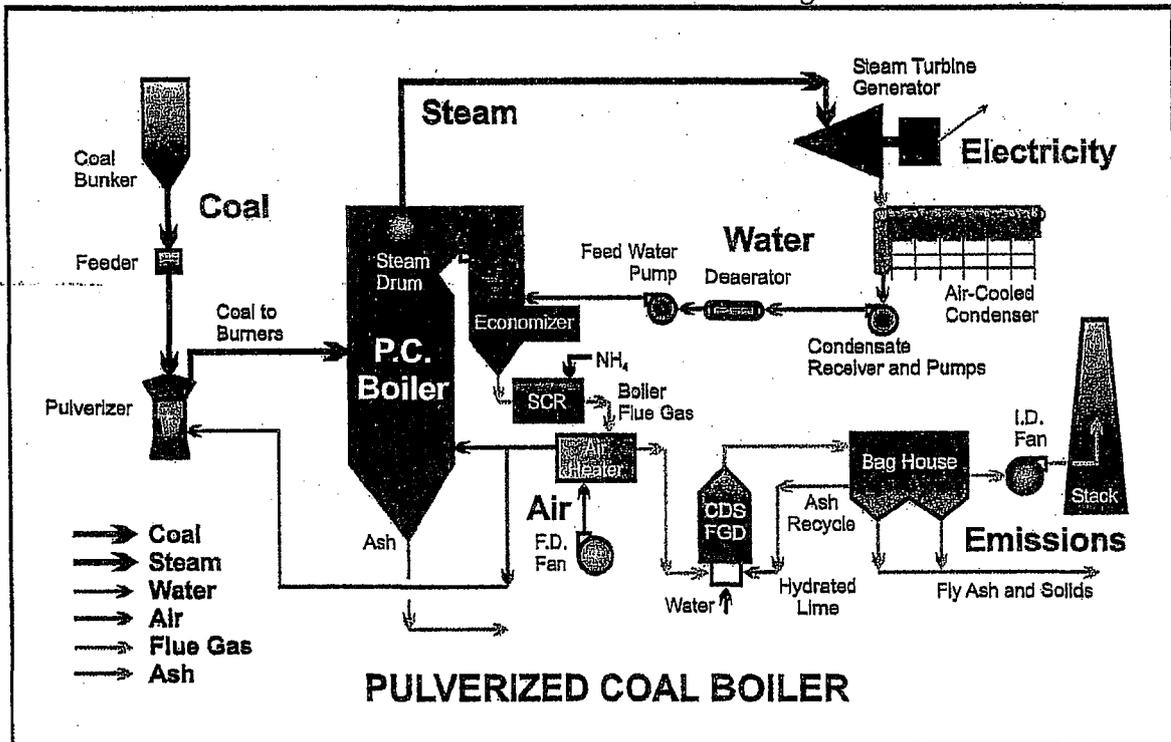
The concept of burning coal that has been pulverized into a fine powder stems from the fact that if the coal is made fine enough, it will burn almost as easily and efficiently as a gas.
