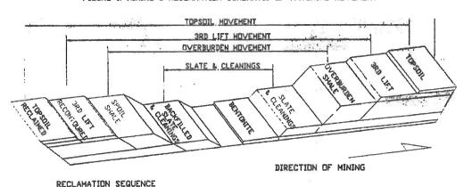
FIGURE 1. MINING & RECLAMATION SCHEMATIC OF MATERIAL MOVEMENT
