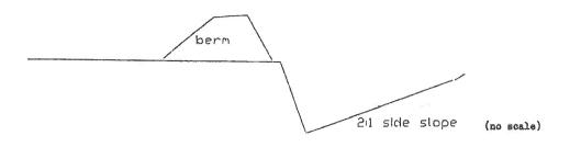
Mine Plan Figure 3. Schematic diagram for trapezoidal channels for diverting ephemeral drainages which watersheds greater than 30 acres
