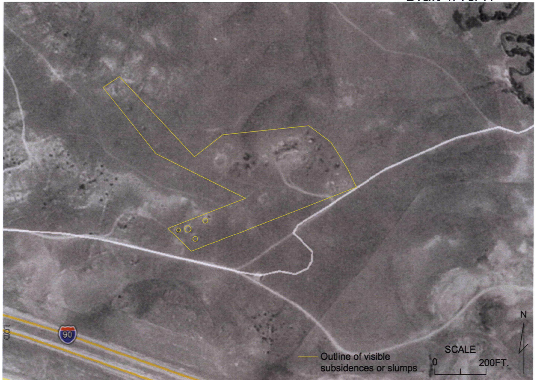
FIGURE 37-3 AREA 2 MINE SUBSIDENCE FROM UNDERGROUND MINING OF THE OLD AGUE NUMBER 3 MINE IN THE UPPER CARNEY SEAM. MINE DEPTH IN THE NOTED SUBSIDENCE AREAS IS 60 TO ABOUT 160 FT. (ADD_D5-4_EX_1_OVB_ISO_R1).
